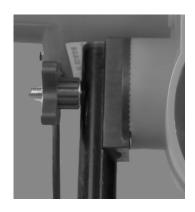
Slide Flat Washer (1st) and Lock Washer (2nd) on to the Long Bolt, then tighten the Knob on to Long Bolt until machine is placed in the desired pitching position.
