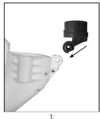
Assemble Ball Feeder Port To Ball Entry End of Machine By Lining Up Holes on Port With Holes on Machine.
